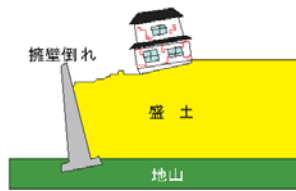
d) 擁壁の倒壊・変状
