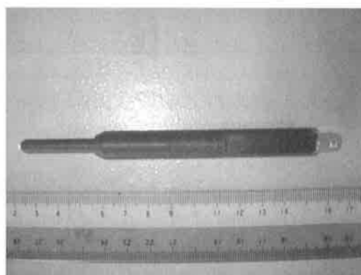
Fig. 2 Magnetic probe (NEC Glass components CP-2S)
