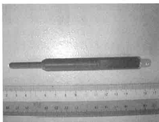
Fig. 2 Magnetic probe (NEC Glass components CP-2S)
