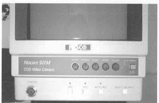
Fig. 15 The example of a trial production of a control panel
