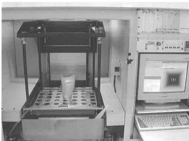
Fig.4 Laser lithography for producing prosthetic sockets
