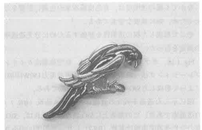
Fig. 4 Deposited transparent protective film on brooch (K18)
